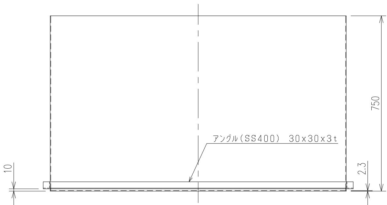
材質: SPHC  $t = 2.3\text{ mm}$
